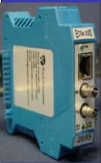
The 2E55 Switched Media Converter Module provides fiber optic conversion to and from wire based Ethernet. The Fiber port operates at 100Mbps and the RJ45 port will auto-negotiate its data rate between 10/100Mbps, Full/Half duplex operation. The 2E55 will automatically learn the addresses of the devices connected to each port (up to 1024) and will buffer and route messages accordingly.
